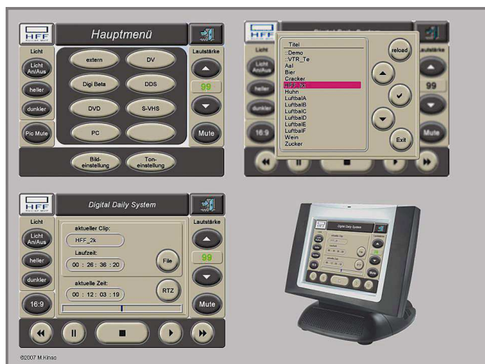
Picture 6. Crestron Touchpanel (picture source: www.crestron.com) and user interface of the HFF Panels (Programming: Mike Kinas, HFF)
